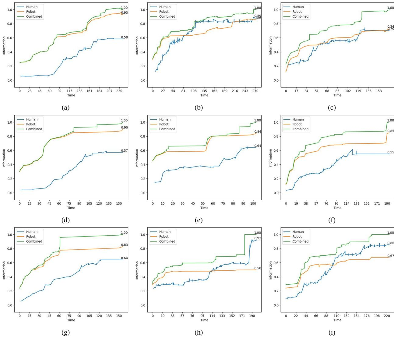
Fig. 6: Information gain results in three different environments (columns  $\{(a),(d),(g)\}$ ,  $\{(b),(e),(h)\}$ , and  $\{(c),(f),(i)\}$ ) for three different strategies (rows): communicating the robots current plan (a)-(c), communicating the exploration state (d)-(f), and communicating the robot's full world model (g)-(i). Note combined information gain is not the sum of human and robot information gain due to overlaps in exploration.
