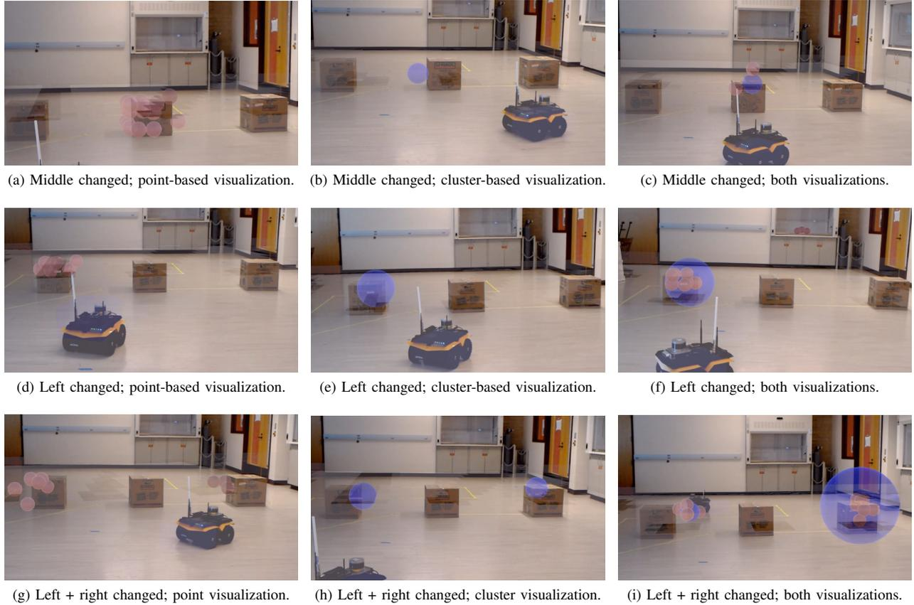
Fig. 2. Examples of the raw point visualization, aggregated cluster visualization, and combined visualization techniques used to indicate the robot’s detected changes in a lab environment, in three different change configurations. In (a)-(c), the middle box changed from the initial model; the left and right boxes were present in the initial model. In (d)-(f), the left box changed. In (g)-(i), the left and right boxes were changes from the initial model.
