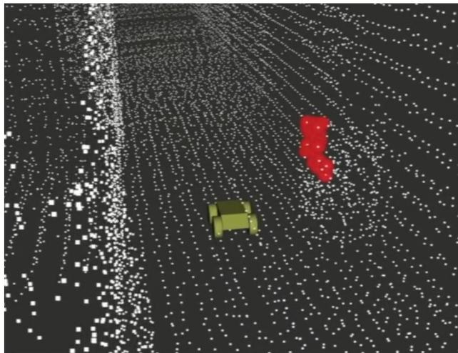
Fig. 1. A robot constructs a relatively dense point-cloud-based map of the environment, and detects changes in the point cloud (shown in red) from a previous reading. This paper seeks to address the problem of how an autonomous robot can convey point-based change detections for interpretation by a human teammate.
