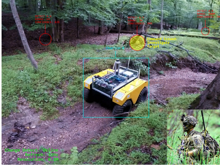
Figure 1: The autonomous robot-based change detection concept. A robot patrols a visually complex environment and conveys information via augmented reality about its position (cyan box) and aggregated change detections (red circles) to a nearby Soldier wearing an AR head-mounted display (inset). The aggregated change detection visualizations support interaction to allow the Soldier to task the robot to further investigate a suspicious change.
