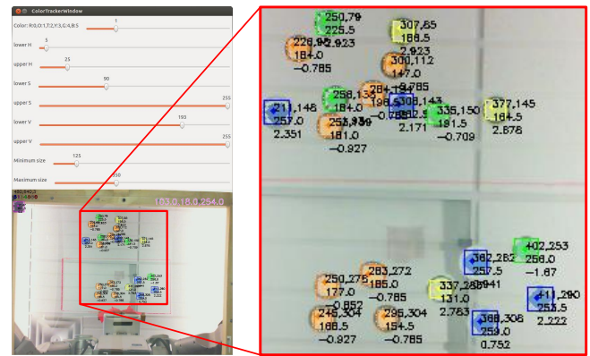
Fig. 6. The object tracker GUI, with live, adjustable parameters on top left and the annotated live image on the bottom left. Right zoom shows an enlarged view of the annotated image. Annotations include position, orientation, size, centroid location, and bounding box for each object.
