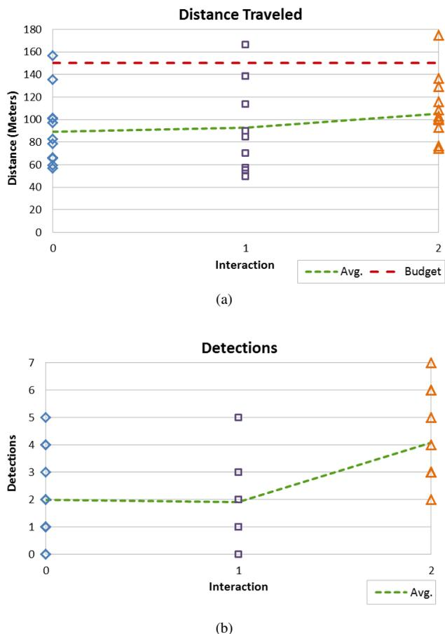
Fig. 7: Experimental results from 34 real-world experiments. (a) shows distance traveled and (b) shows target detections out of 10 possible targets.
