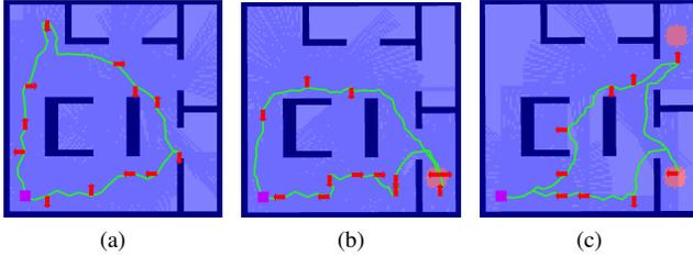
Fig. 4: Example of the effect of interaction on route surveillance generation in a complex environment. (a) shows the baseline case, where a route is generated autonomously with a uniform target distribution. (b) shows the impact of a single interaction, where a route after the target distribution prior is modified to elevate an area of higher target probability, shown as the red circle. (c) shows the autonomous route generated after two interactions.
