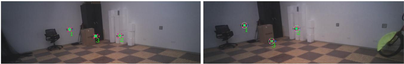
Fig. 5: Snapshots of the JPDAF tracking three quadrotors at two time instants. The pink crosses represent the measurement (detection), the bold green circles show the tracks positions (with their corresponding ID), and the thin green ellipsoids around each track show the position covariance in the image space.
