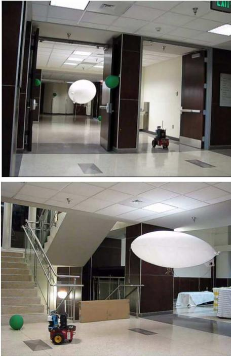
Fig. 4. On the top, the UAV waits on the ground robot for localization assistance. On the bottom, the robot assists the UAV in localizing a target.
